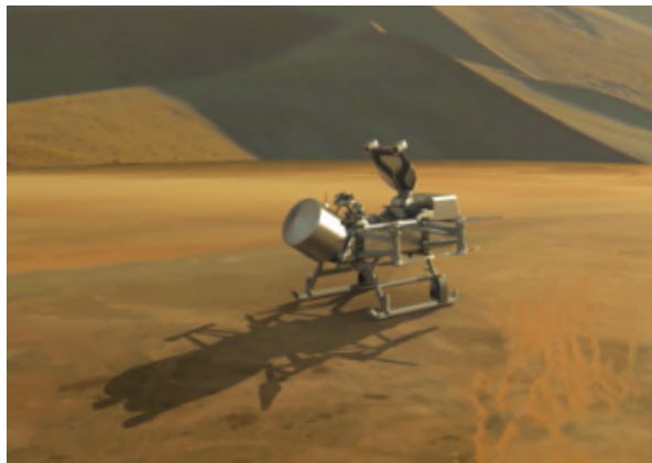
Figure 1: The Dragonfly lander sitting on an interdune plain: the MMRTG is the cylinder at left, and the high gain antenna is deployed for direct-to-Earth communication. Each skid features a sampling drill and sensors to measure surface properties.
